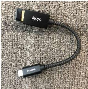
b. Insert the Dongle to the USB port located on the short side of the tablet. The LED on the USB Dongle should blink green when it is plugged in
