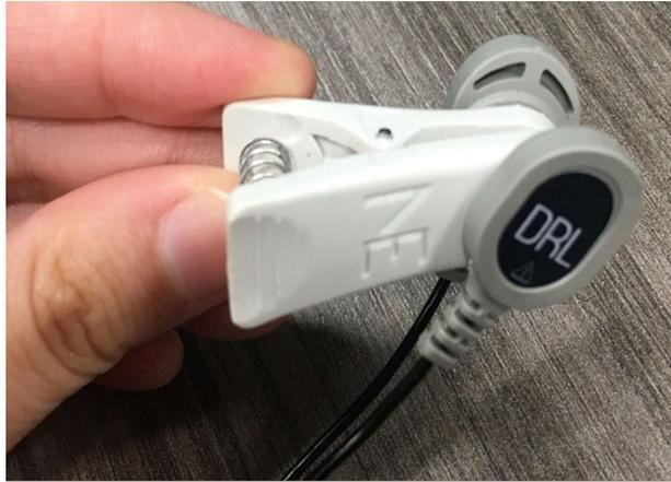
j. Secure the earclip onto the participant's right earlobe. Make sure the earclip does not slide off from the earlobe.
